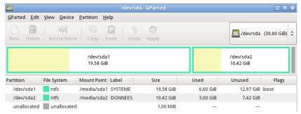
*Figure 3: Source disk geometry, before shrinking partitions*
