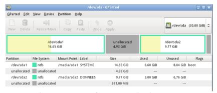
Figure 4: The new geometry after partition shrinking
